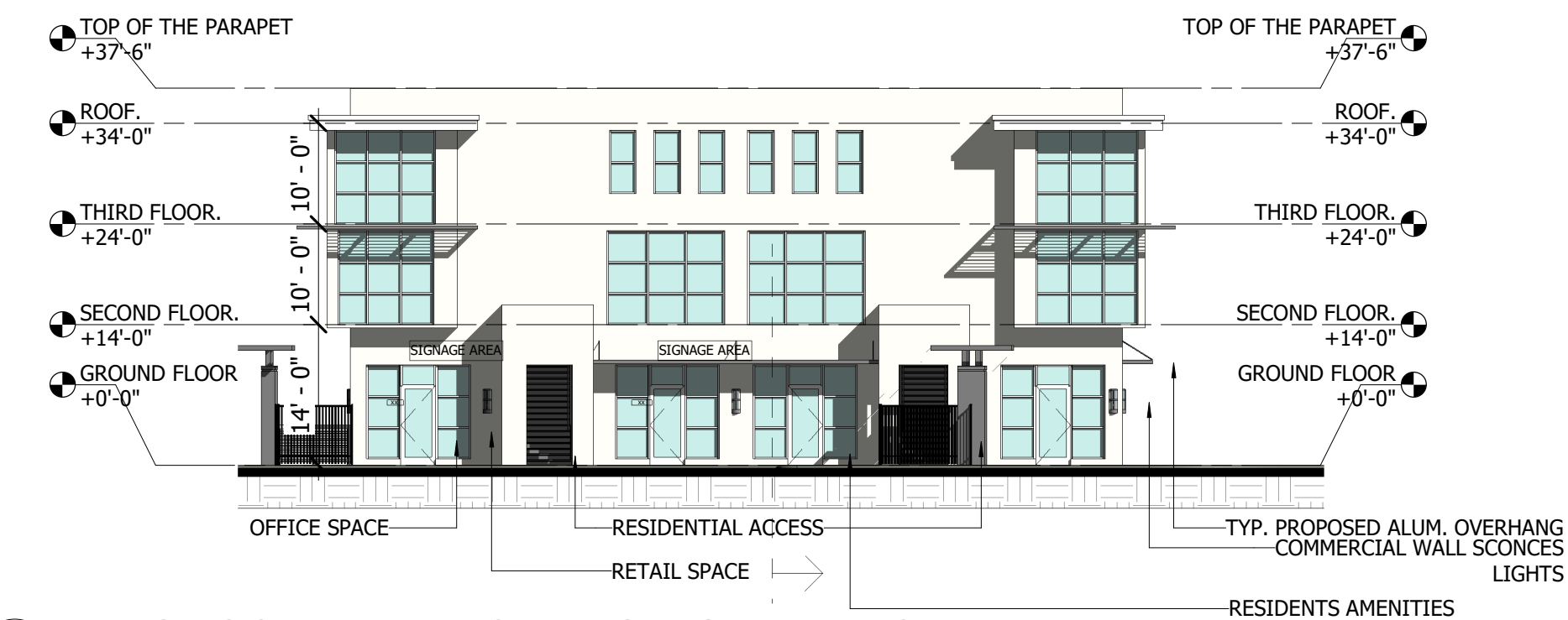
4 BLDG 1&3 - ELEVATION FACING INTERIOR PLAZA SCALE: 1/16" = 1'-0"
