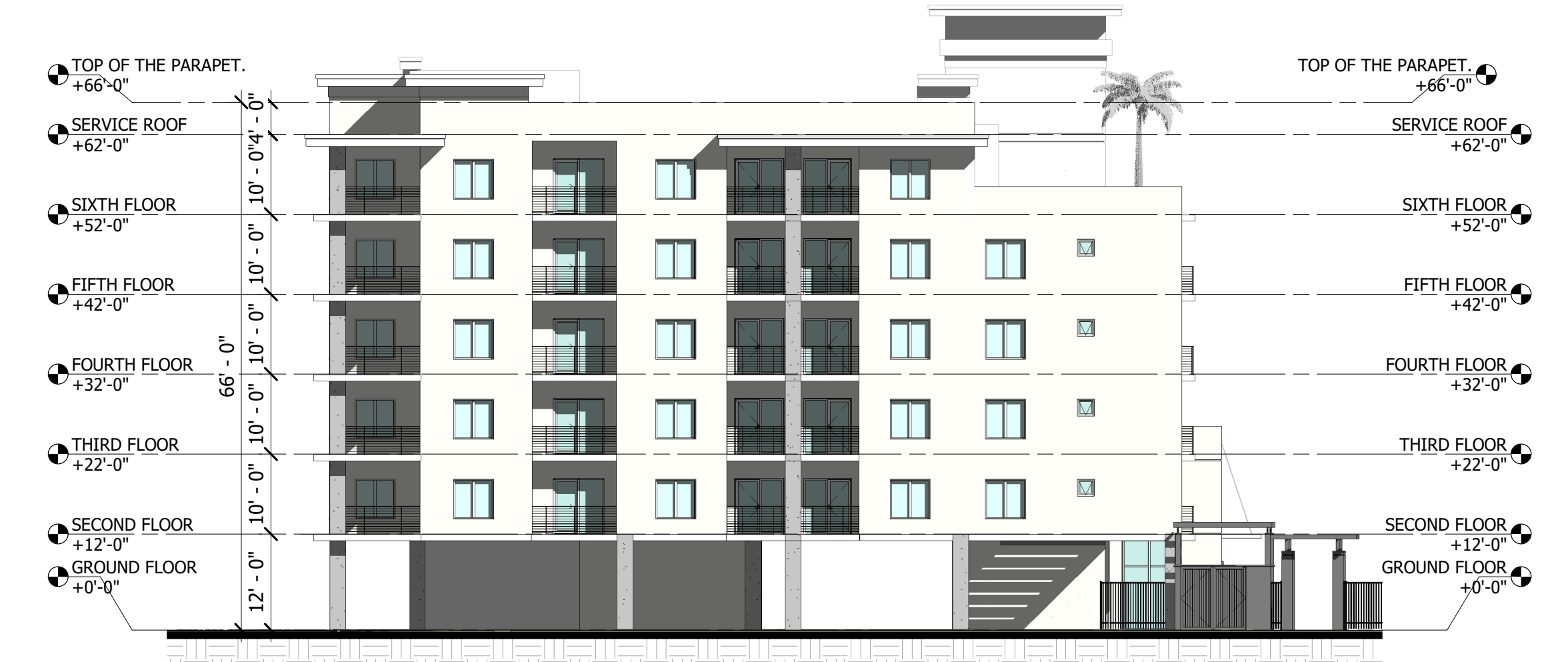
4 BLDG 2 - SOUTH ELEVATION SCALE: 1/16" = 1'-0"
