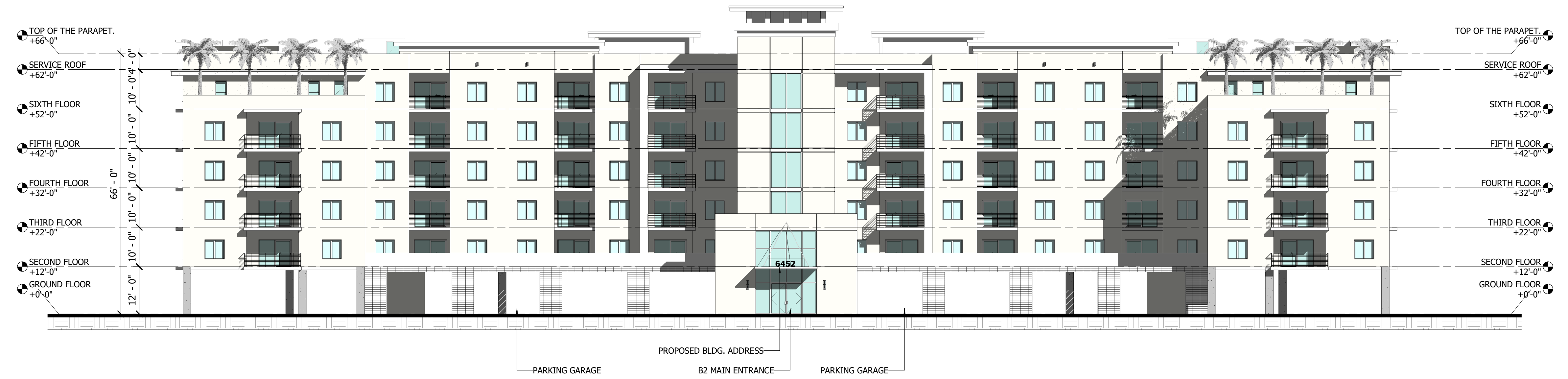
1 BLDG 2 - EAST ELEVATION SCALE: 1/16" = 1'-0"
