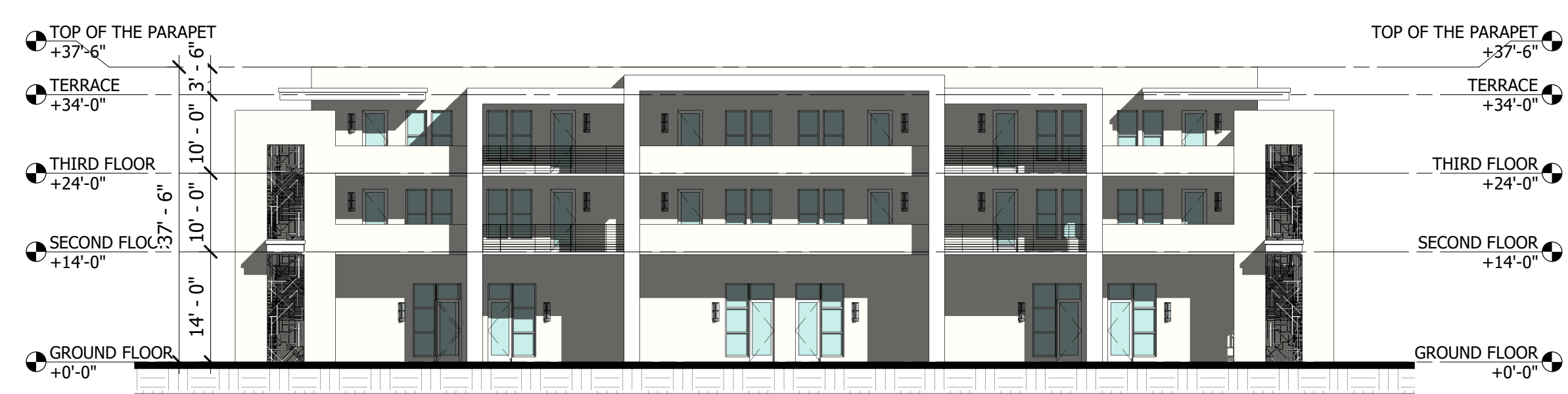
3 BLDG 4 - WEST ELEVATION FACING INTERIOR PLAZA SCALE: 1/16" = 1'-0"
